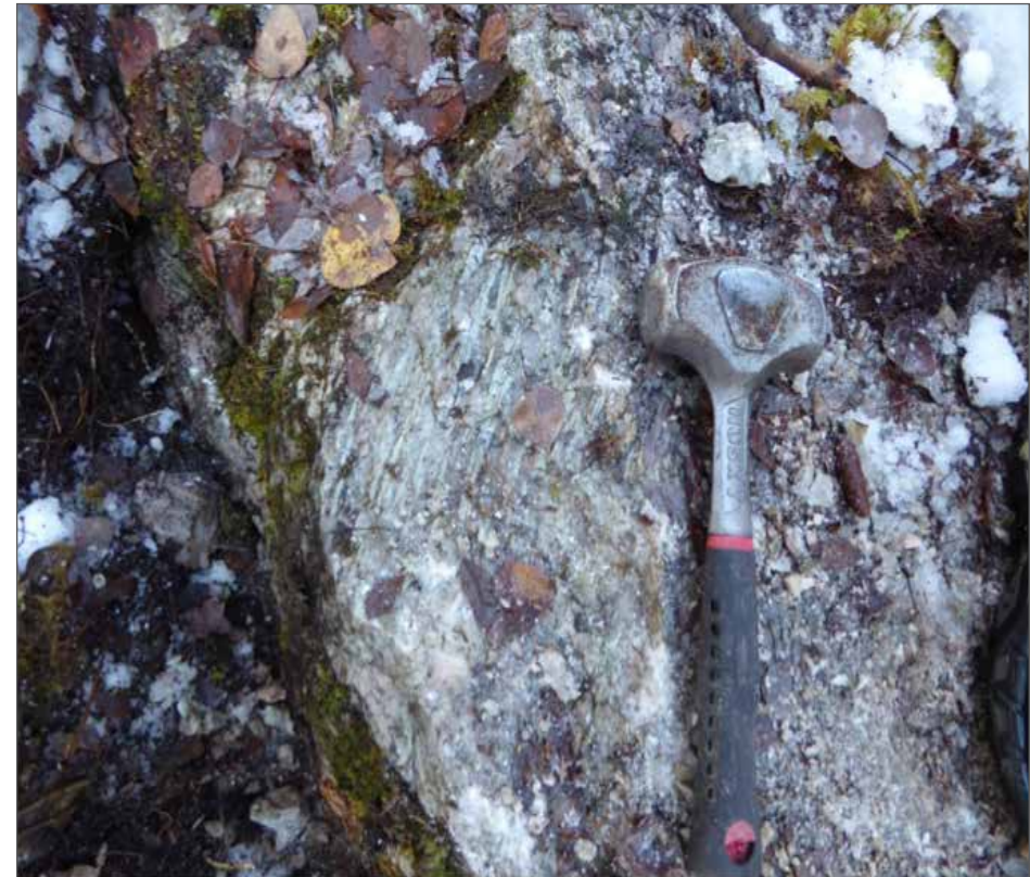
Sample 099701 – Spodumene clusters in pegmatite (7,520ppm Lithium, 1.62% \text{Li}_2\text{O} )
