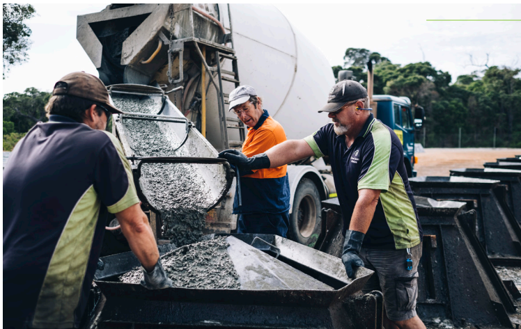
MAKING THE ABITATS: Pouring cement into our custom built abitats - specifically designed and tested as a habitat for the greenlip abalones.
