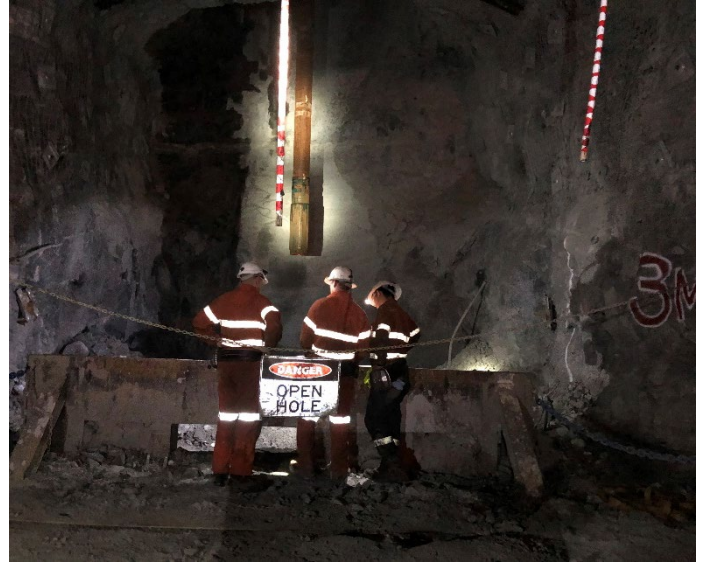
Figure 3: Rods being lowered from the surface to 1675 RL
