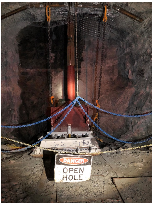
Figure 4: Reamer head connected to rods
