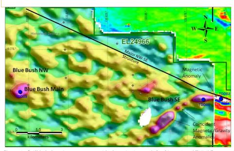
Figure 1 - Drill hole location map over residual gravity image (left of image) and TMI 1VD magnetic image ( right of image).
