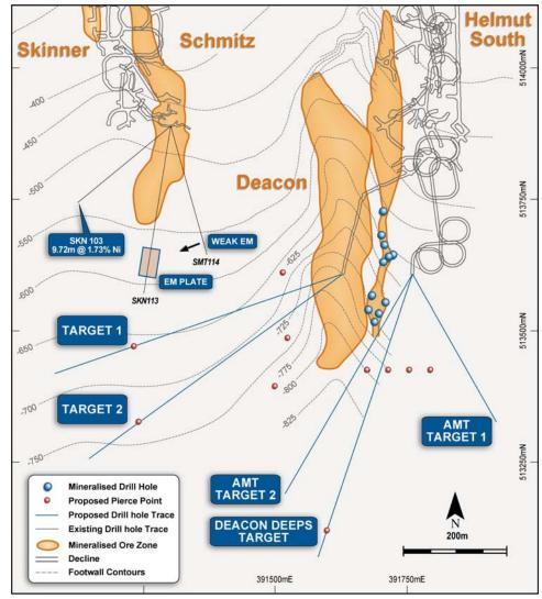
Figure 2: Schimtz/Deacon extension drilling plan
