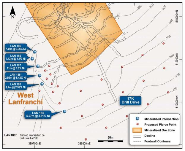
Figure 3: Lanfranchi Channel extension drilling
