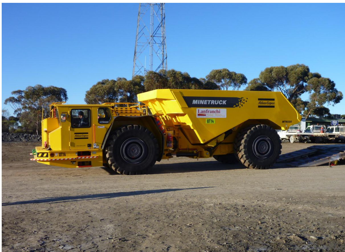
Photo 1: New Atlas Copco MT6020 underground truck (60t capacity) delivered to the Lanfranchi Project in July 2012
