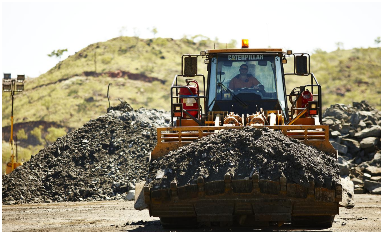
Photo 2: Savannah Run-of-Mine (ROM) Loader taking a bucket of nickel ore to the Process Plant crusher
