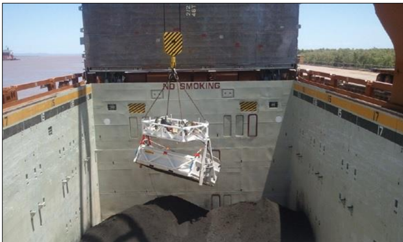
Photo 1: Tipping Jig loading Savannah concentrate into a ship's hold at the Port of Wyndham
