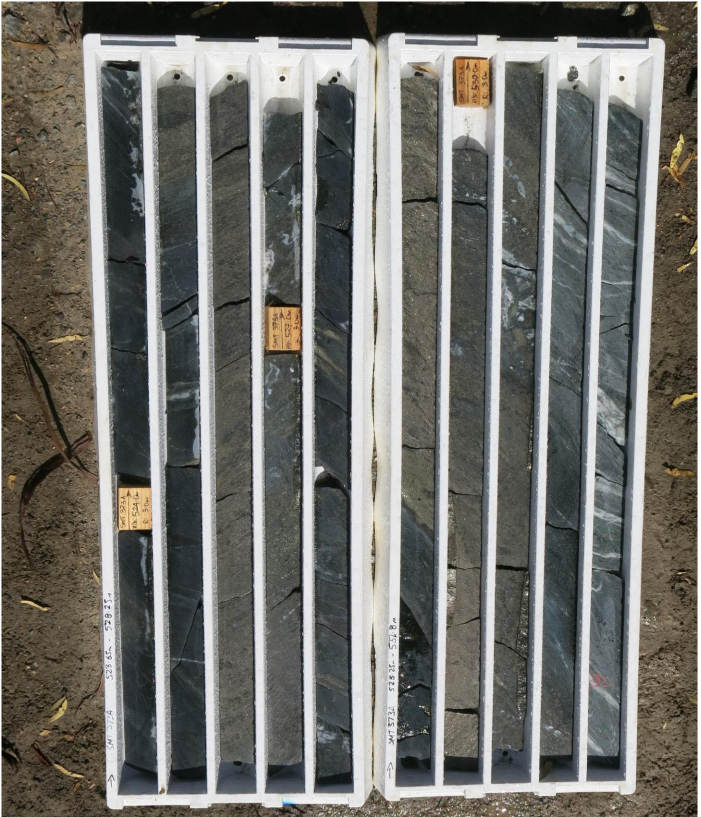
Photo 2 – Drill core from SMT373A intercept from 525.30m (6.80m @ 5.02% Ni)
