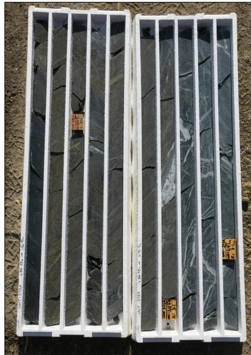
High-grade drill core from SMT373A intercept from 482.90m (6.10m @ 5.73% Ni)
