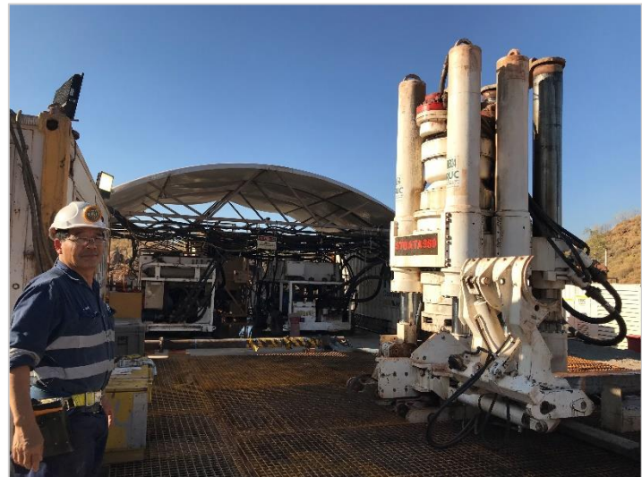
Savannah North raise bore rig and platform
