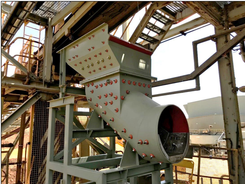
Photo 3 - New SAG mill feed chute
