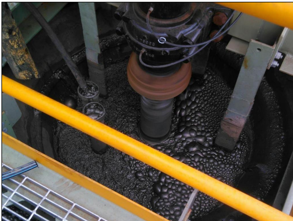
Photo 4 - Flotation cells in operation
