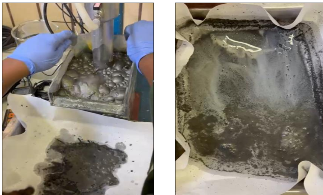
Figure 5: Copper Flotation Test (left) and Copper Rougher Concentrate (right)
