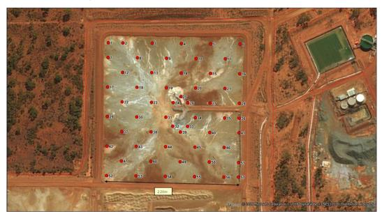
Figure 1: Plan view of 2018 sonic drilling showing collars for resource definition and metallurgical holes
