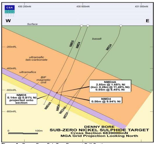
Figure 3: Denny Bore-Sub Zero Prospect Drill Section
