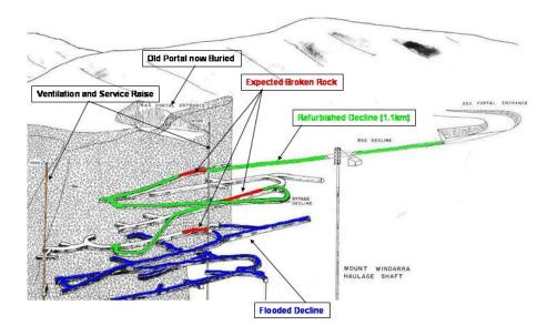
Figure 2: Long Section showing rehabilitation progress of the Mt Windarra mine decline
