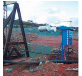
In June 2010, Poseidon restarted the dewatering program at the Mt Windarra underground mine. In the 16 months that the pumps were out of action during the GFC, the water level only rose by 40 metres.
