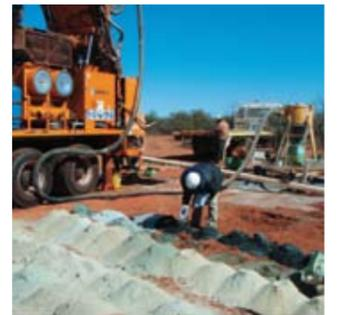
A geologist is seen here testing rock chips using a Niton XRF gun. The Niton gives geologists a much quicker insight into the presence of nickel and other metals, saving several weeks waiting for laboratory assays and greatly improving the flexibility of the drilling program.
