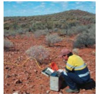
The discovery of 7 well defined lava channels led to the redeployment of Electromagnetic testing at Windarra. Rather than broad testing, the Company was able to focus on individual locations to prioritise the drill program.
