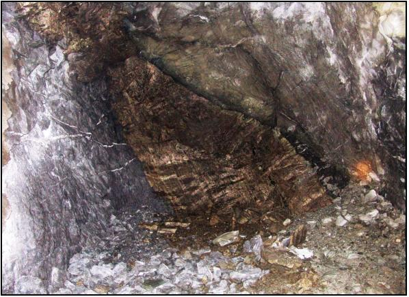
Figure 3: Goose 10170 level (now mined) showing high grade massive nickel sulphide (~13% Ni) in the ore drive.
