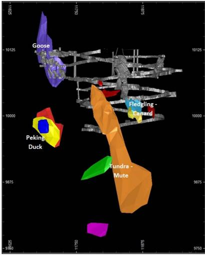
Figure 1: Long section looking west of the in situ lodes at the Silver Swan deposit
