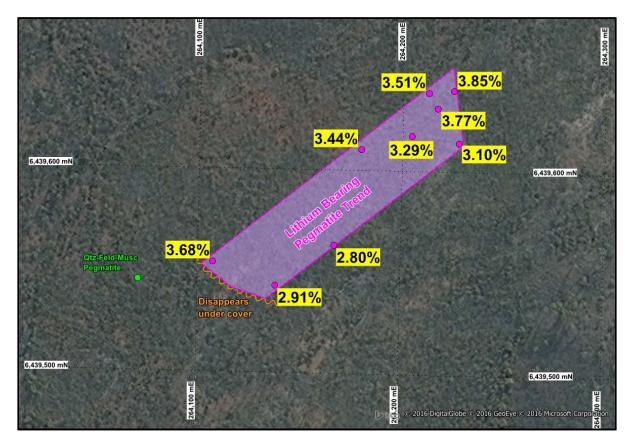
Figure 2: Location of sampled lithium bearing pegmatite with Li<sub>2</sub>O% assay results
