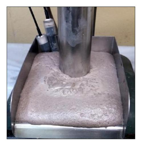
Figure 3: Pegmatite flotation test
