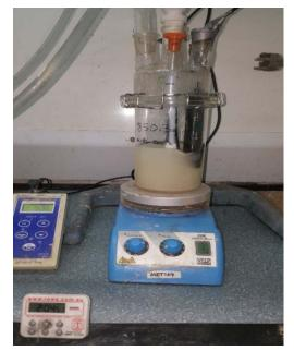
Figure 6: Lithium Hosted Pegmatite Leaching Research Equipment
