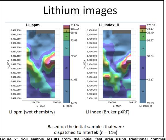
Figure 2: Soil sample results from the initial test area using traditional commercial laboratories methods versus a calibrated Bruker pXRF machine programmed to calculate lithium using propriety Lithium Index estimation. Results returned an 89% correlation.
