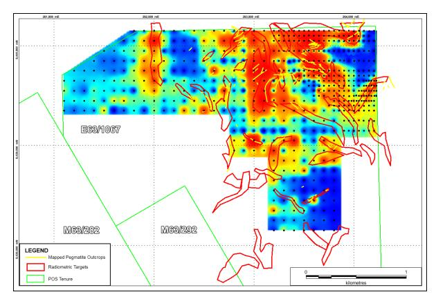
Figure 3: Identified radiometric anomalies coincide with lithium soil sampling anomalies as well as highlighting new unsampled target areas
