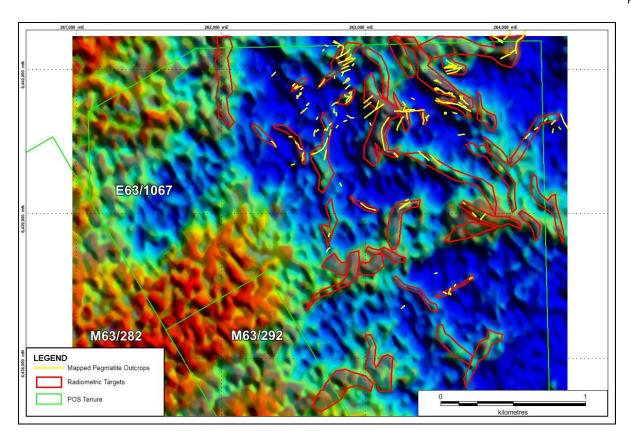
**Figure 2:** Potassium and total count radiometric anomalies define multiple strong anomalies (red outlines) which coincide with known mapped pegmatites (yellow lines) as well as additional anomalies in the south
