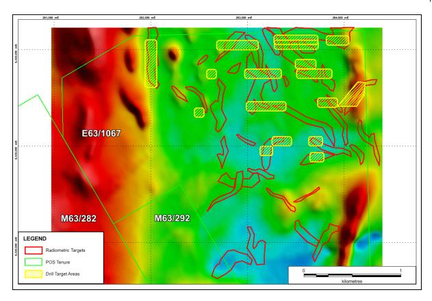
Figure 4: Drill targets (yellow hatched areas) overlie TMI image and the coincident defined radiometric-soil anomalies
