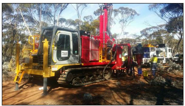
**Figure 6:** Core Drilling Services RC drill rig is mounted on a rubber tracked X300-Morrooka base which can traverse the hilling/rocky terrain with minimum environmental impact.
