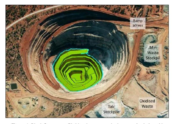
Figure 4: Black Swan open Pit (development at the bottom of existing pit)
