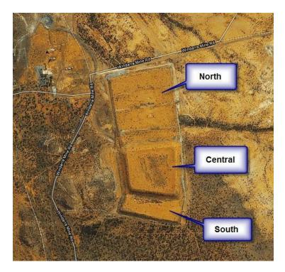
Figure 1: Configuration of the Tailings Dams at Windarra
