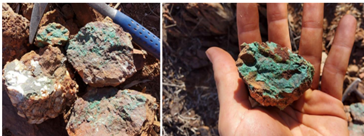
Figure 1 – Samples containing malachite (green) at the Scimitar Target indicating the presence of copper.
