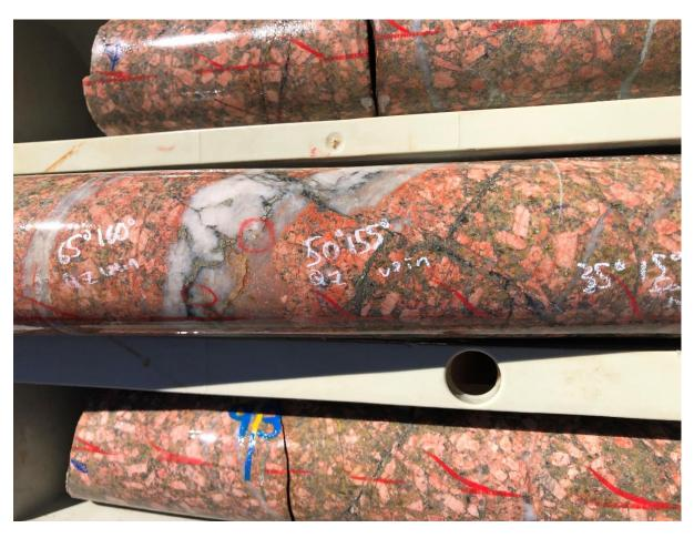
Figure 5 – HQ diamond core from BCDD2101 containing quartz veining with sulphide and visible gold in altered monzonite at 92m downhole
