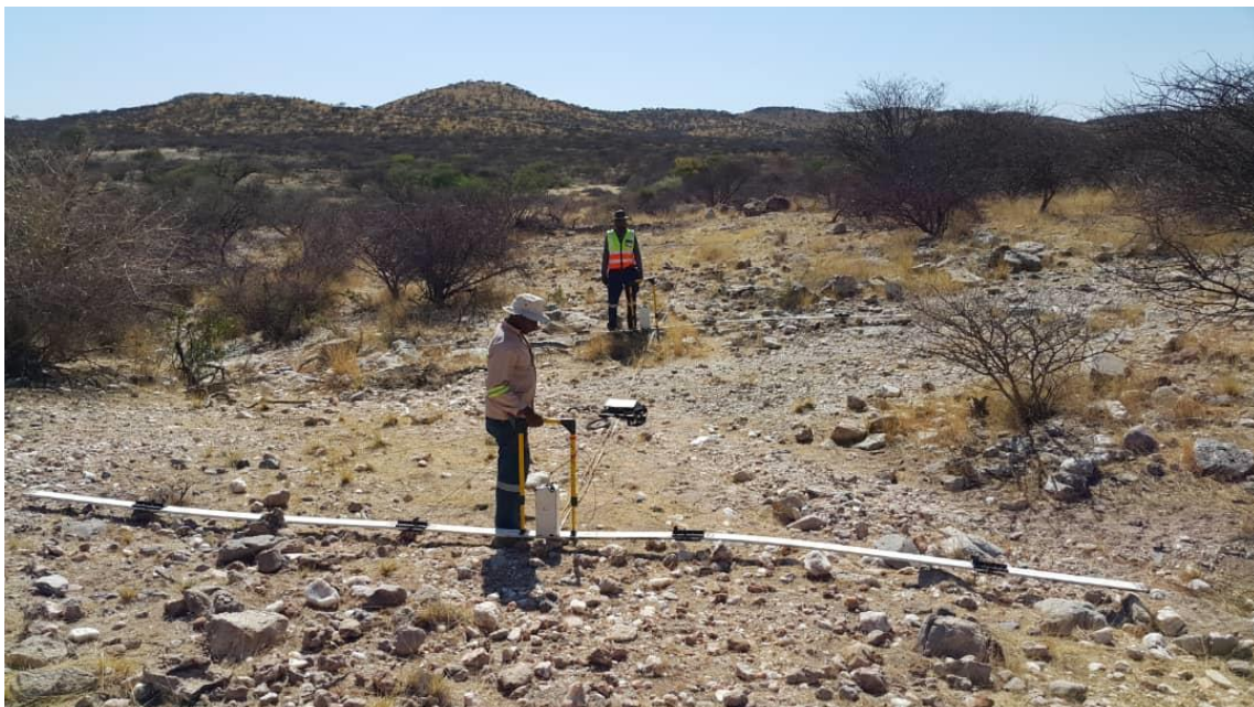
Figure 2. GPR survey work in progress
