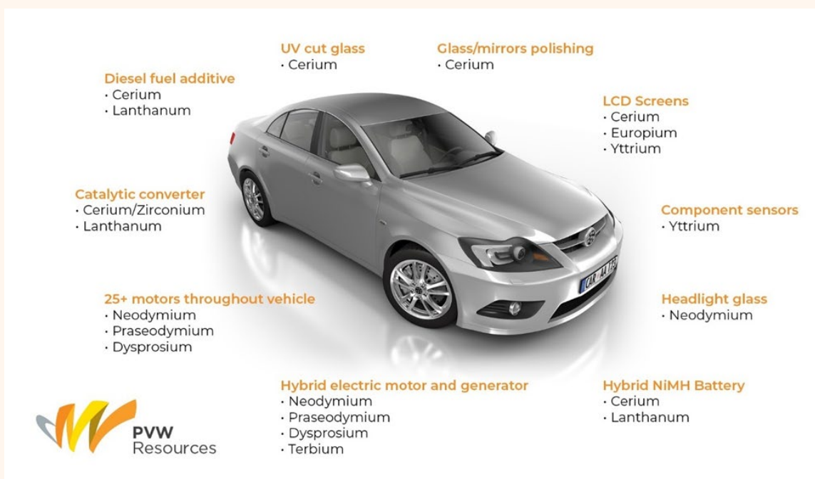
Figure 3: Rare earth elements used in electric vehicles
