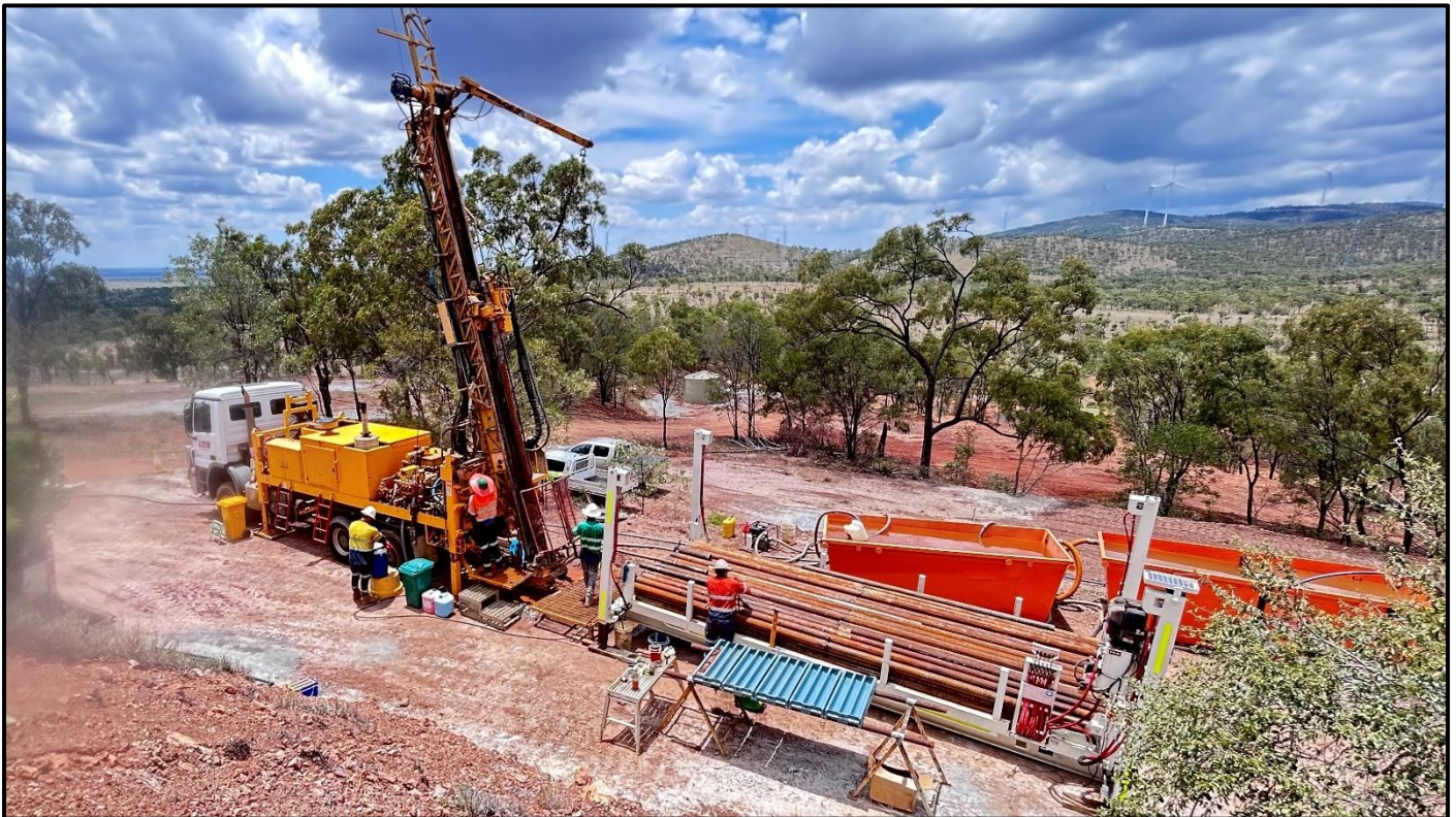
Figure 1: United Drilling's UDR650 drilling MMDD007 at the North Knoll deposit
