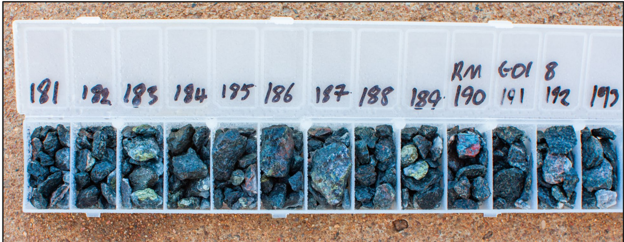
Figure 3. Chalcopyrite-pyrite sulphide zones at Mongoose – RMG018 181 – 193 m.
