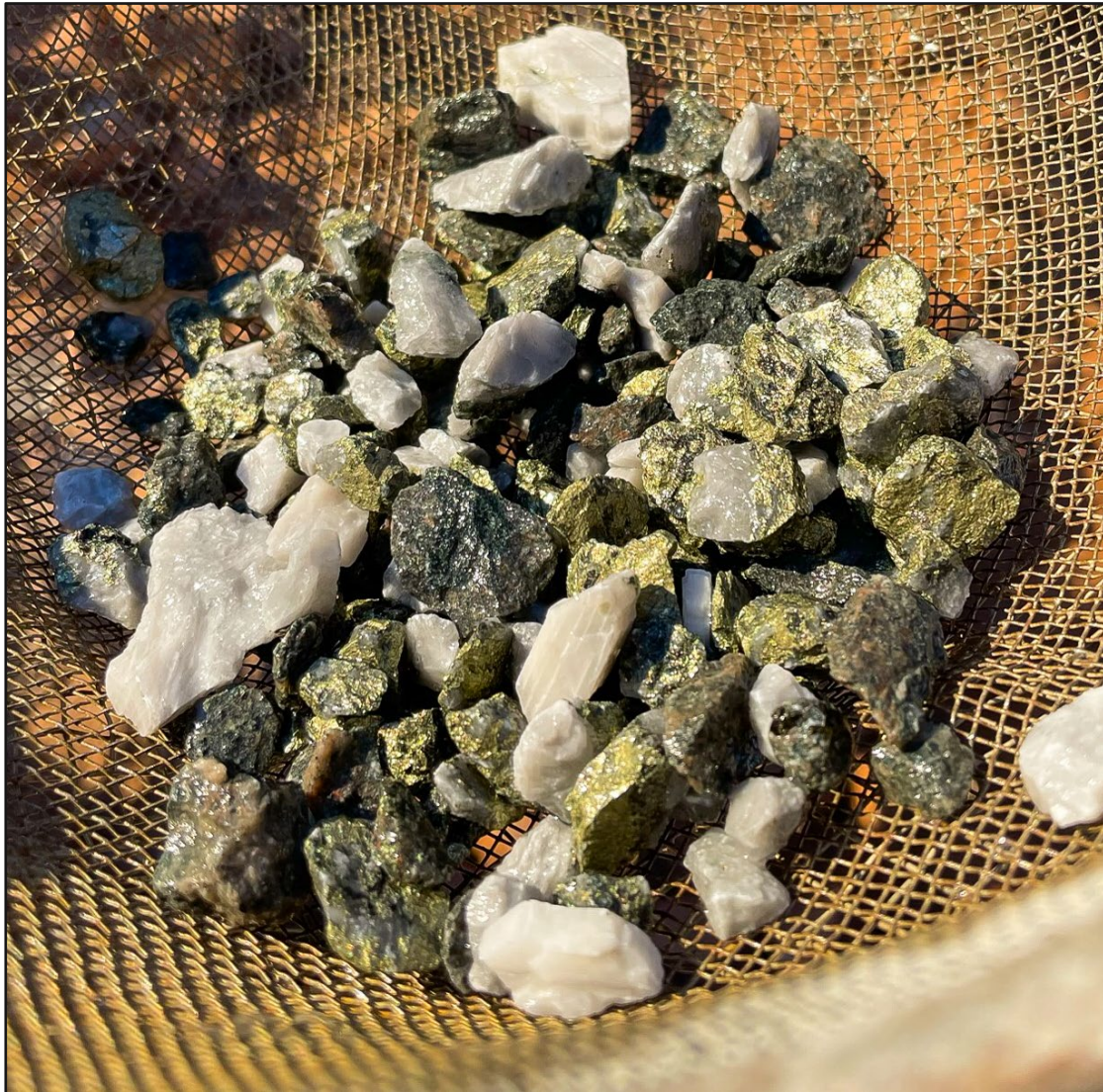
Figure 1. Chalcopyrite-pyrite sulphide mineralisation at Mongoose - Hole RMG032, 119-120 m.
