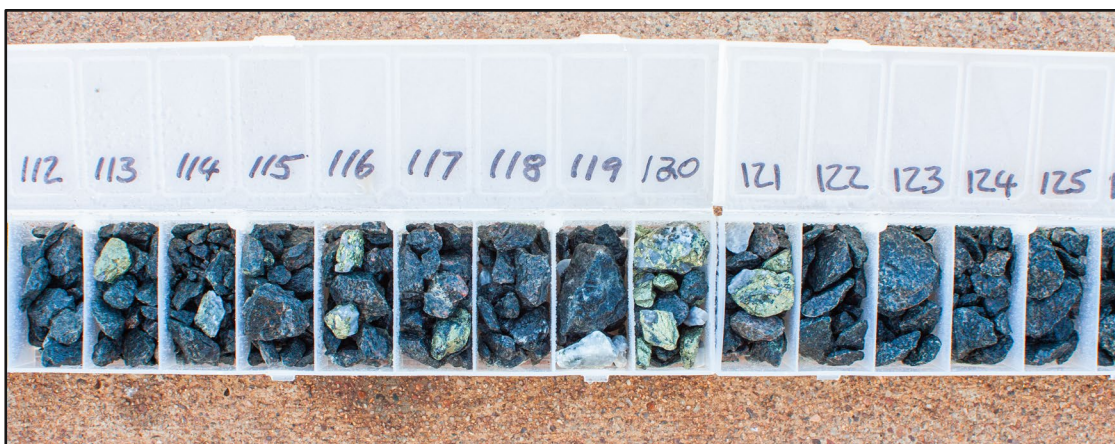
Figure 2. Chalcopyrite-pyrite sulphide zones at Mongoose - Hole RMG032, 112 – 125 m.
