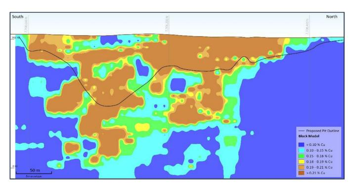
Figure 3. Mongoose Resource cross section showing smoothed optimised pit and block model heat map (447937E)
