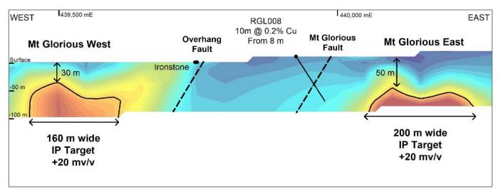
Figure 9. Mt Glorious Prospect, showing cross section of the processed IP dipole-dipole survey, looking north.
