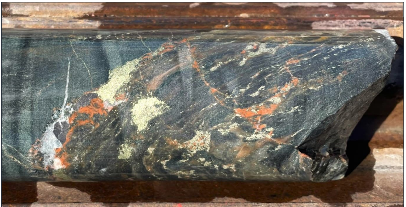
Figure 5: RMD001, showing a shear zone with magnetite, biotite, red rock, chalcopyrite and pyrite, at 306m down hole. (See Table 2)
