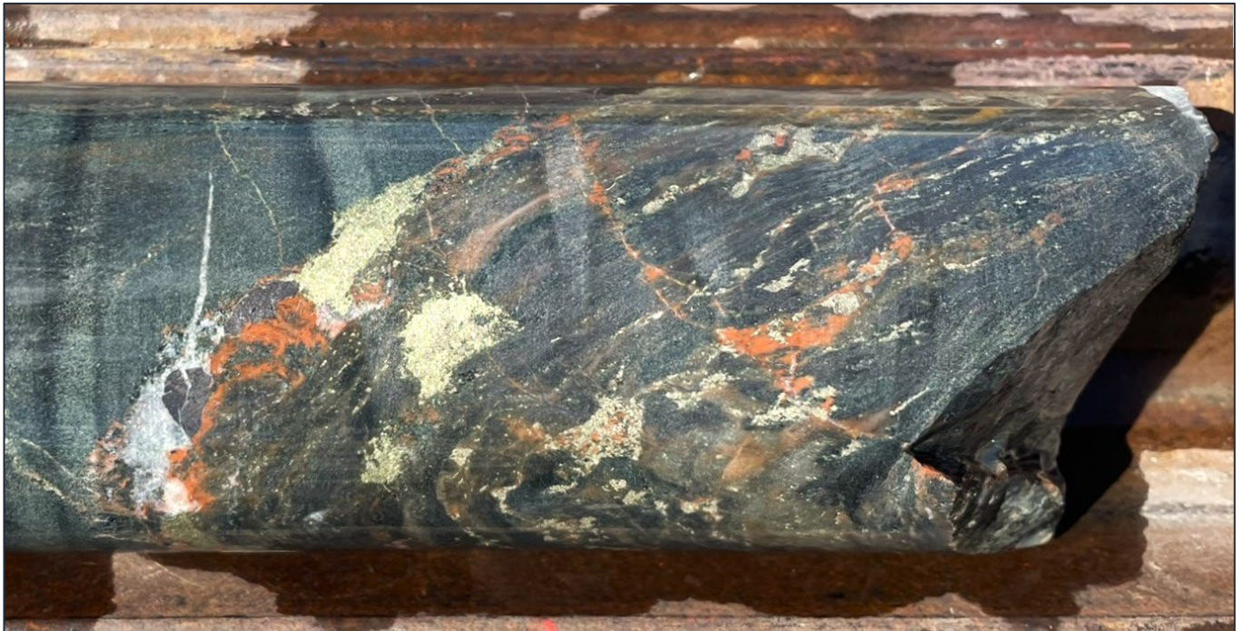
Figure 7: RMD001, showing a shear zone with magnetite, biotite, red rock, chalcopyrite and pyrite, at 306m down hole.
