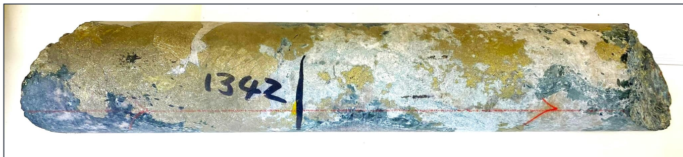
Figure 3: RMD001 pyrite, calcite, chalcopyrite vein, at 1342m down hole. 5
