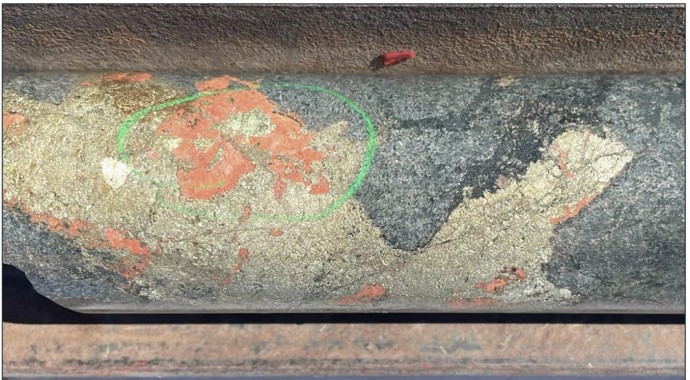
Figure 7: RMD001 breccia zone showing massive pyrite, red rock and chalcopryite, at 532.5m down hole. 5
