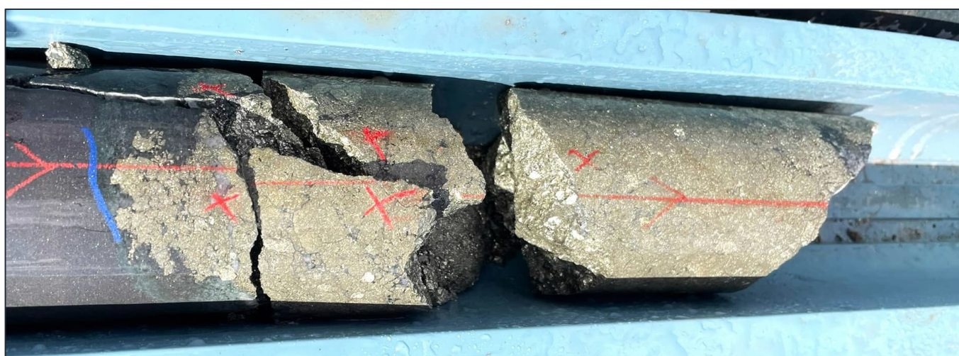
Figure 4: RMD001 massive pyrite, at 212m down hole. 5
