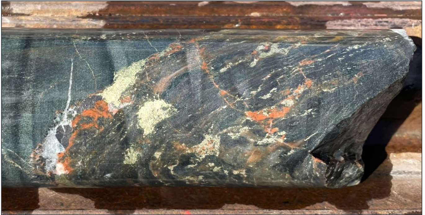
Figure 6: RMD001, showing a shear zone with magnetite, biotite, red rock, chalcopryite and pyrite, at 306m down hole. 5
