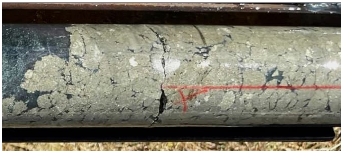
Figure 5: RMD001 massive pyrite, at 316m down hole. 5
