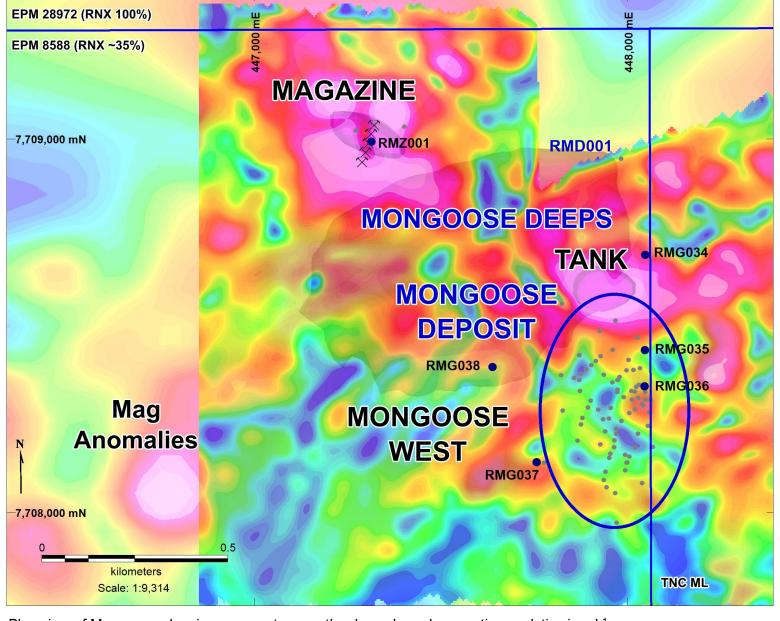
Plan view of Mongoose showing prospects upon the drone-based magnetics analytic signal.<sup>1</sup>
