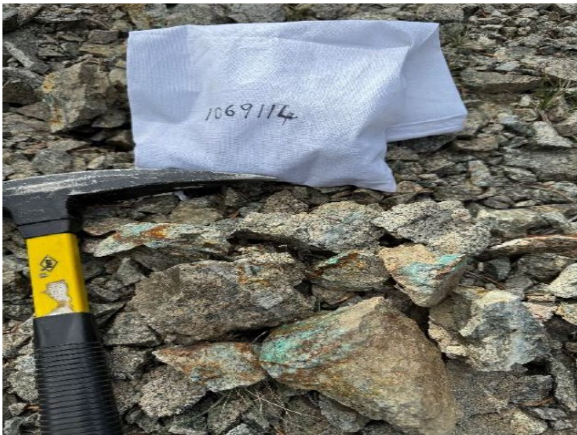
Figure 3. Sample 1069114 - Porphyry-type C-type quartz stockwork
