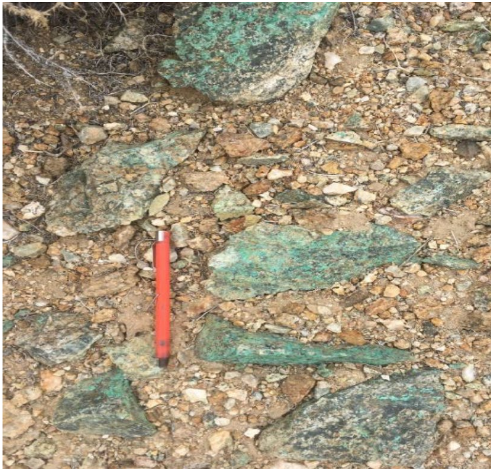
Figure 6. Altered granodiorite in sample 587240 (>1.0% Cu) (Refer ASX Release 10 June 2025)
