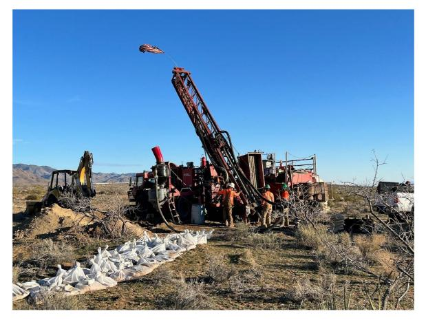
Figure 2 – RC Drilling at Tintic - March 2022
