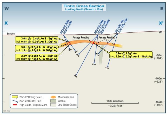
Figure 1 – Tintic Cross Section X-X'
