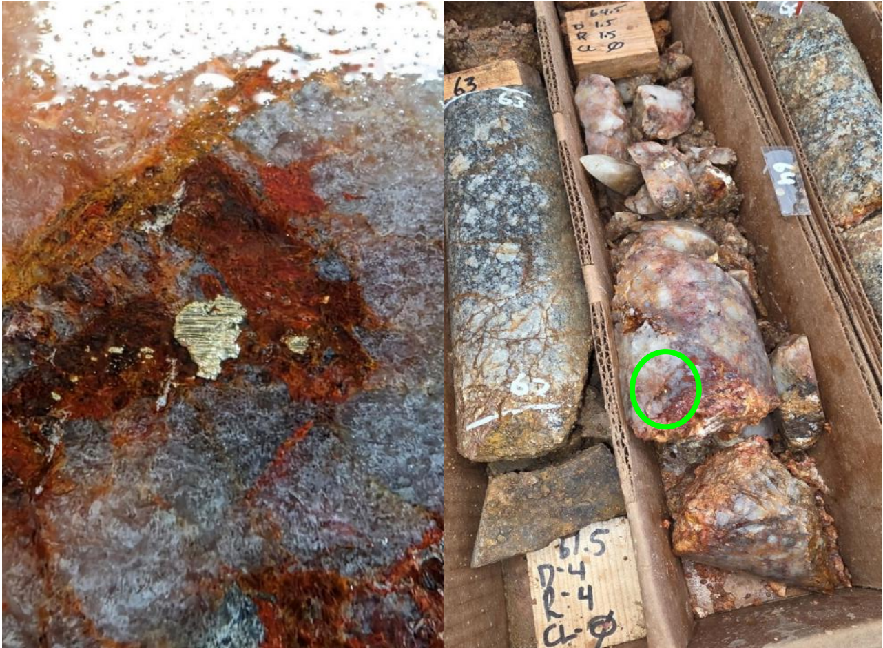
Figure 4: ~30 cm of a massive quartz-sulphide (30%) vein returned 0.61m @ 71.9 g/t Au, 92.5 g/t Ag from 19.2m. Oxidation of sulphides to goethite–limonite–hematite with native gold preserved as ragged/leafy grains spatially associated with the iron-oxides.
