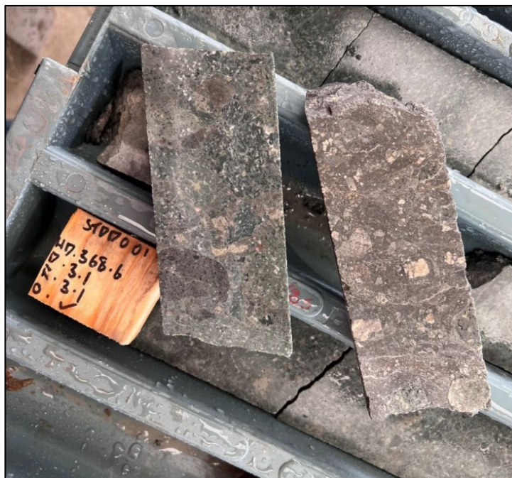
Photo 1. Poly-phase hydrothermal breccia with mineralised clasts and clasts of sulphide (mainly pyrite but some minor galena noted) in a rock-flour/fine pyrite/carbonate matrix – STDD001 HQ3 diameter ½ drill core~ 368m drill depth.
