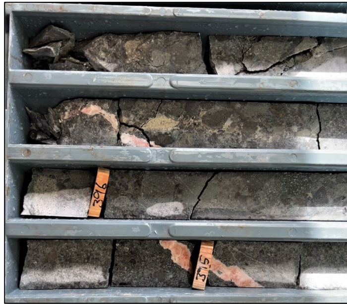
Photo 2. Poly-phase hydrothermal breccia with mineralised clasts and clasts of sulphide (mainly pyrite but some minor galena noted) in a rock-flour/fine pyrite/carbonate matrix – with cross-cutting pink Mn-carbonate rhodochrosite veins - STDD001 HQ3 diameter ½ drill core ~ 395m – 398m drill depth.
