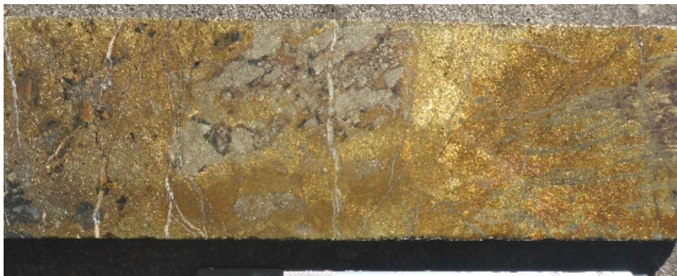
Figure 3: DTD002: 481.2m which includes a 0.67m interval of massive chalcopyrite + pyrite + minor bornite, in quartz magnetite brecciated vein – sample assayed 25.6% Cu & 1.29g/t Au.
