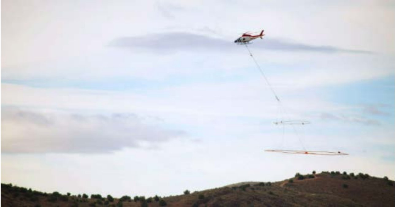
Figure 3: VTEM Max helicopter-borne AEM system in operation.
