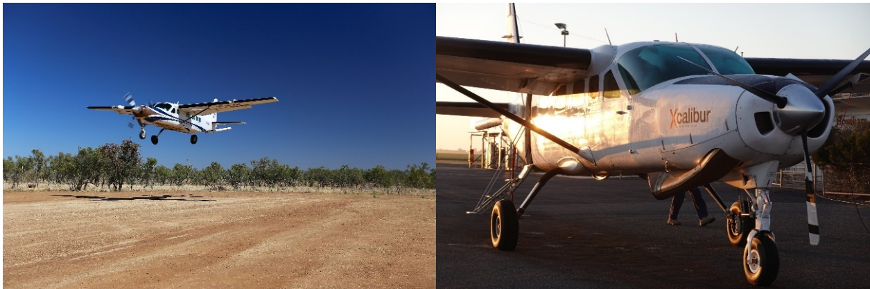
Figure 1: FALCON AGG system on a Cessna C208 Grand Caravan aircraft.
