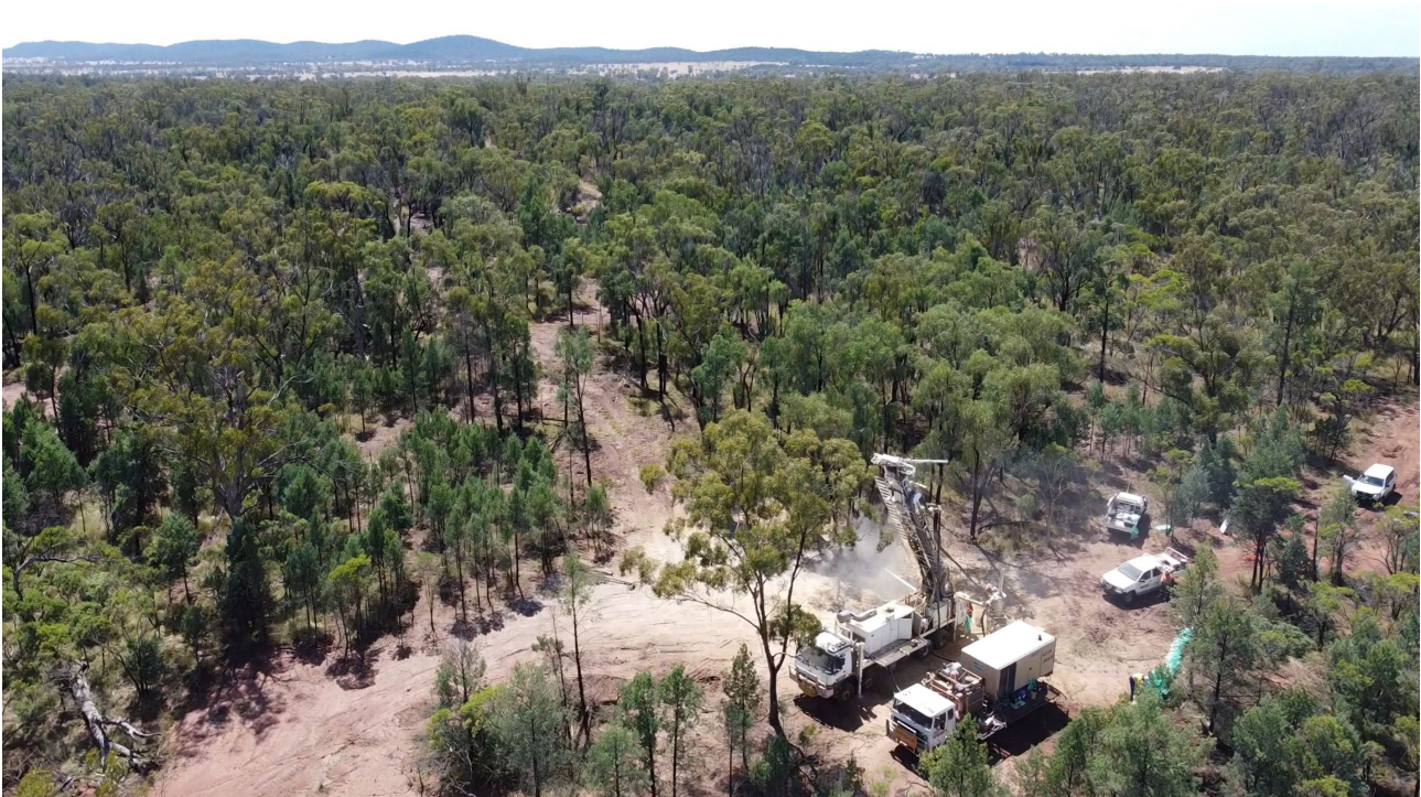
Figure 1 – RC drilling in progress at the Carpina North gold prospect.
