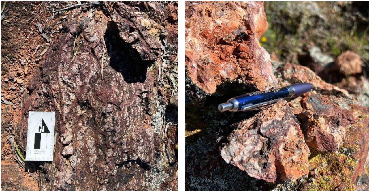
Figure 7 - North-south striking quartz veining on EL8659 and Fe-Mn staining associated with boxworks ex-sulphide.
