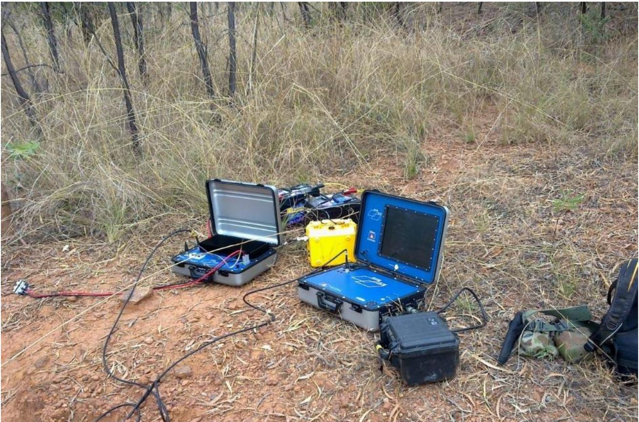
Figure 4 – Fender Geophysics MLEM receiver equipment in-field.
