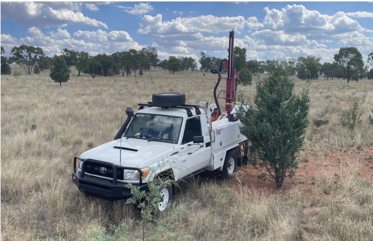
Figure 2 – Talisman's in-house auger drill rig.
