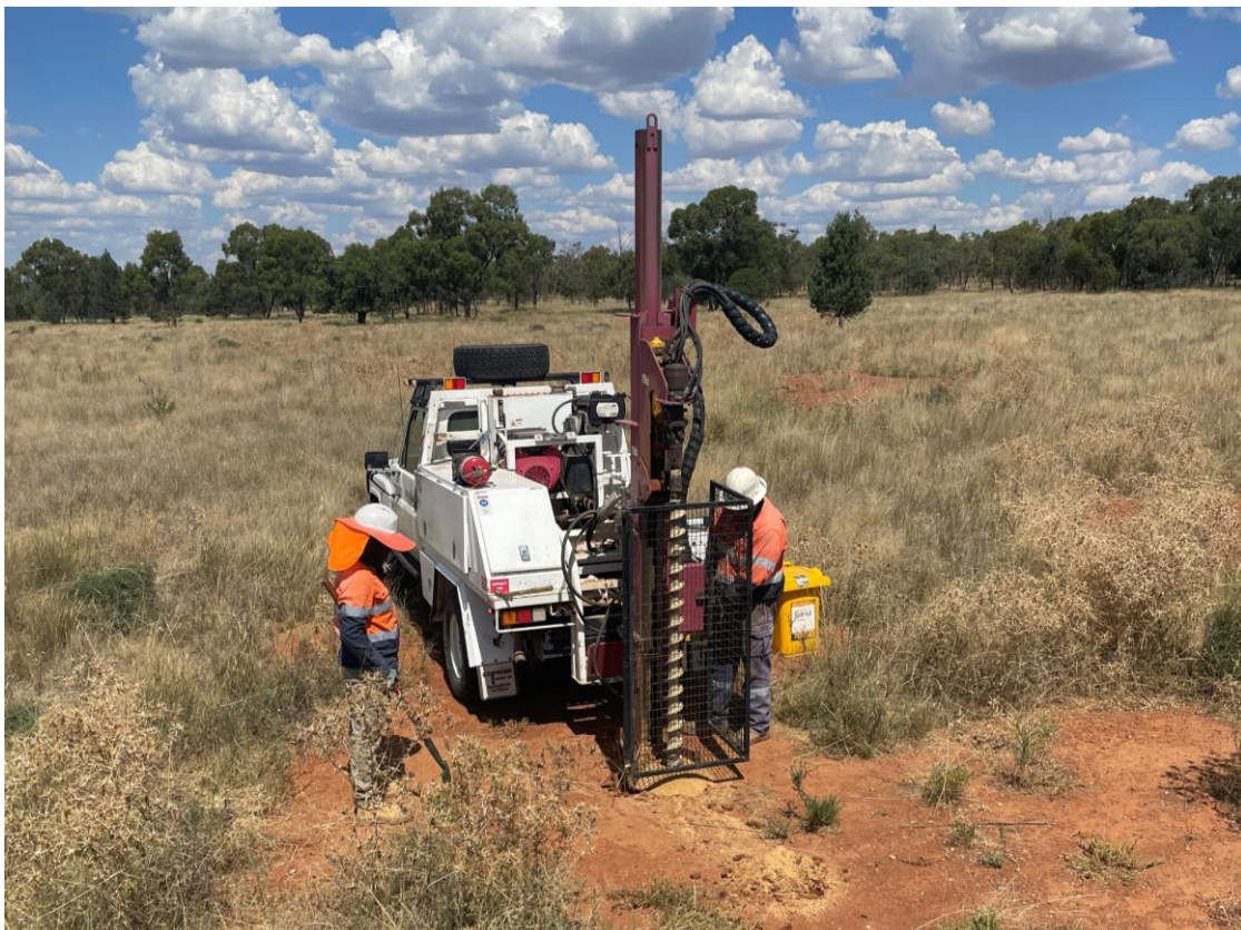
Figure 1 – Auger drilling in progress on Exploration Licence 8571.
