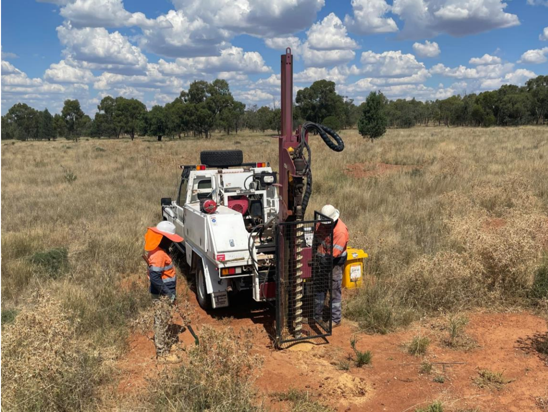
Figure 3 – Auger drilling in progress on EL8571.
