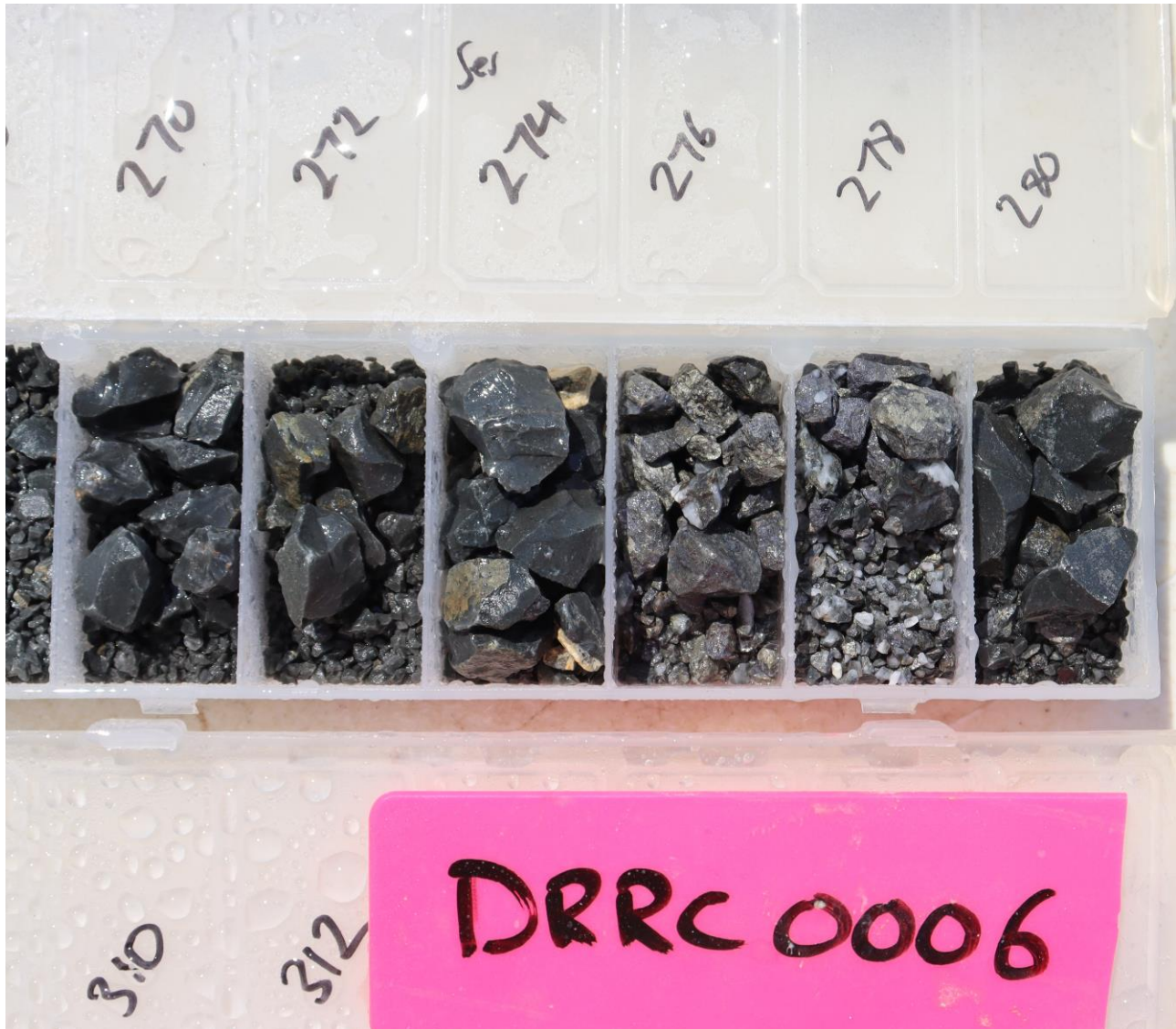
Figure 4 – Durnings RC chip tray closeup from DRRC0006, 270m-280m. The 6m section from 274m to 280m shows significant sulphide mineralisation coincident with 10.3% Pb, 3.5% Zn, 126g/t Ag, 0.4% Cu and 1.93g/t Au. Fine sulphide mineralisation is logged throughout the intersection with quartz sulphide breccia logged from 274-280m.
